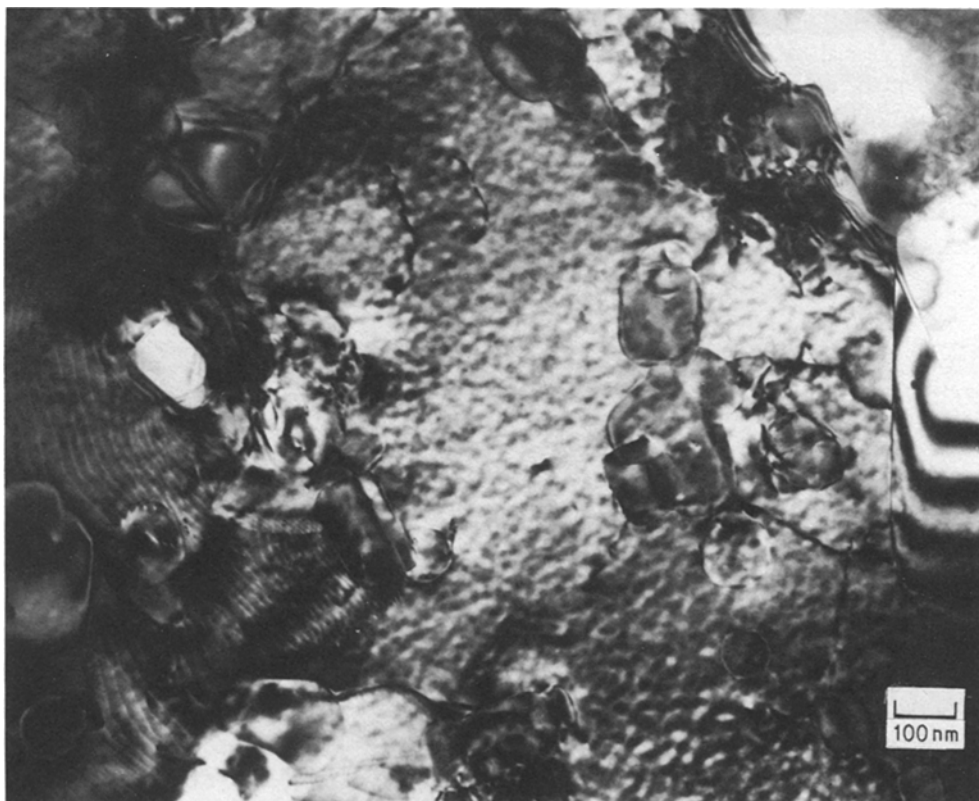
Figure 8 Region from within Fig. 7 showing agglomeration of small beryllium particles as a result of consolidation.
